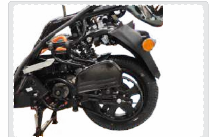
Mid mount motor with belt drive
