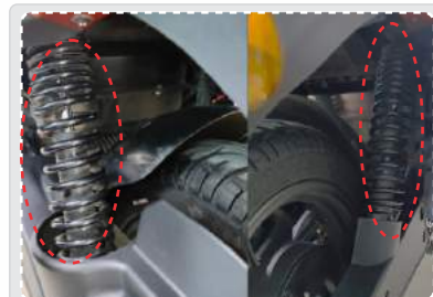
Twin rear suspensions for safe shock absorption and comfort
