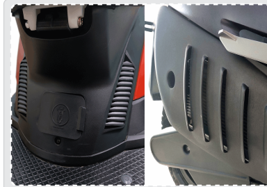
Air vents for cooling of the electrical parts
