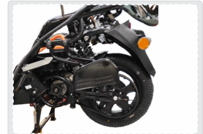
Mid mount motor with belt drive
